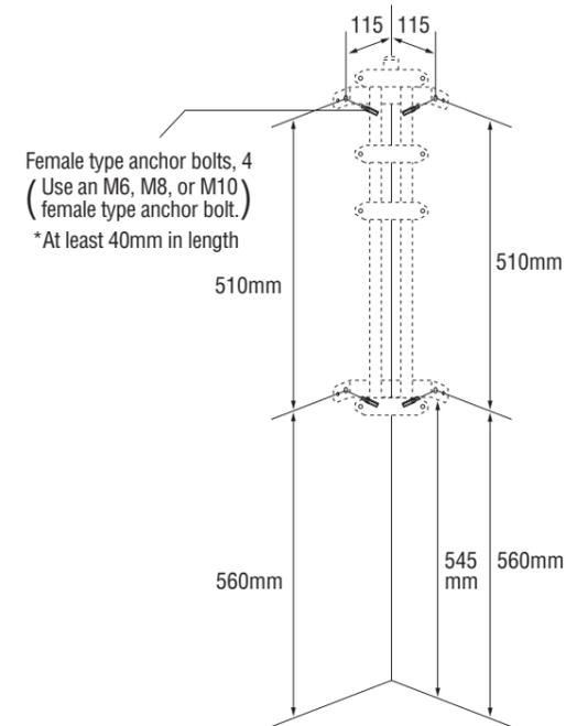
**3** Fix the corner fixtures to the wall at four mounting points.
