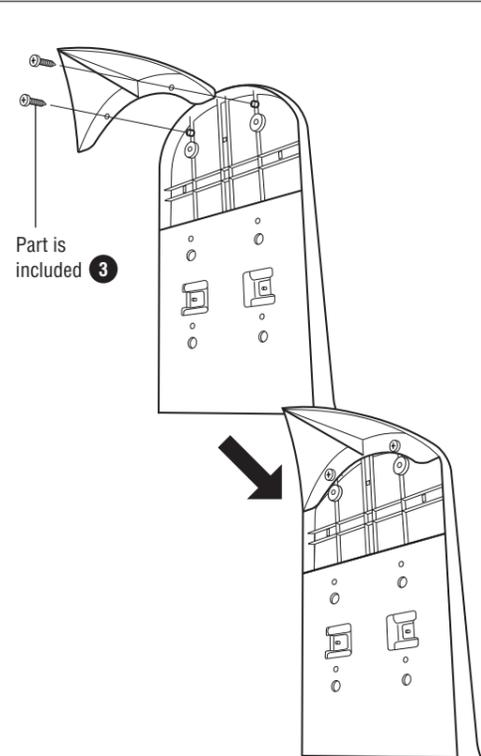
**6** Attach the base to the corner fixture connected to the wall.
