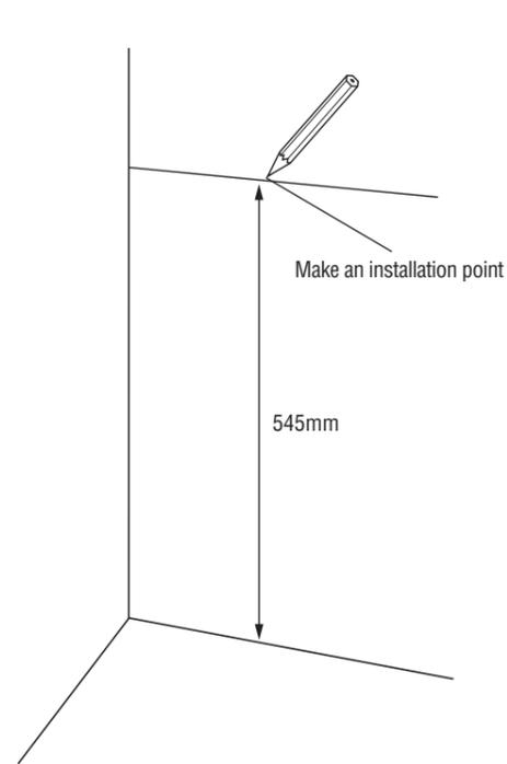
**2** Align the bottom points of the corner fixtures to the areas marked on the wall. Once four points have been marked on the wall, install the anchor bolts.
