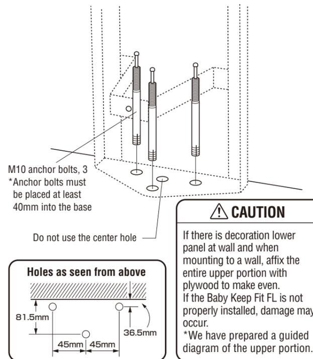
**3** Return the base to its original location as indicated above, and fix the Baby Keep Fit FL to the floor at three mounting points.
