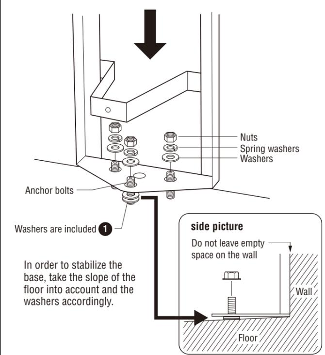
**4** Fix the Baby Keep Fit FL to the wall at four mounting points. (Refer to "Types of Screws Used for Wall-mounting" on the other side of this instructions)
