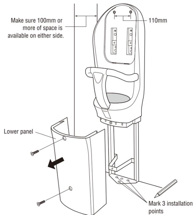
**2** Remove the base, and screw in the three anchor bolts where indicated.
