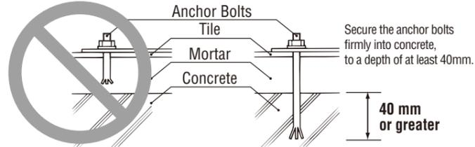
Secure the anchor bolts firmly into concrete, to a depth of at least 40mm.
