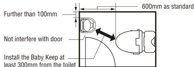
• Install on a wall at least 600mm away from the toilet, or insure 300mm of space between the Baby Keep Fit FL and toilet.
