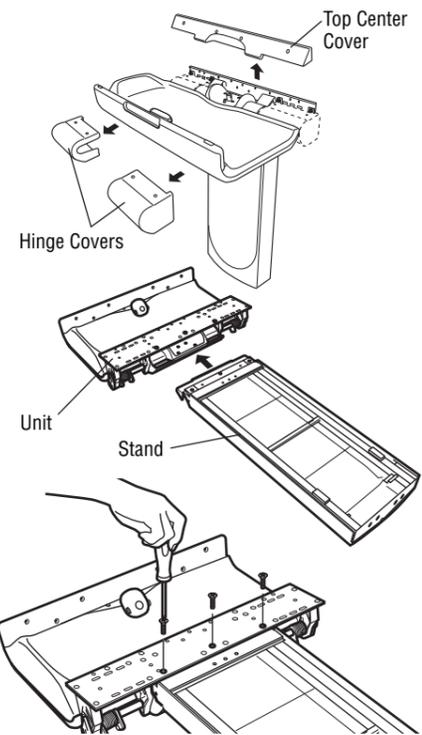
**2** Remove the two (2) screws from the stand cover and then remove the stand cover. Confirm where the stand cover attaches and make a mark to indicate this.
