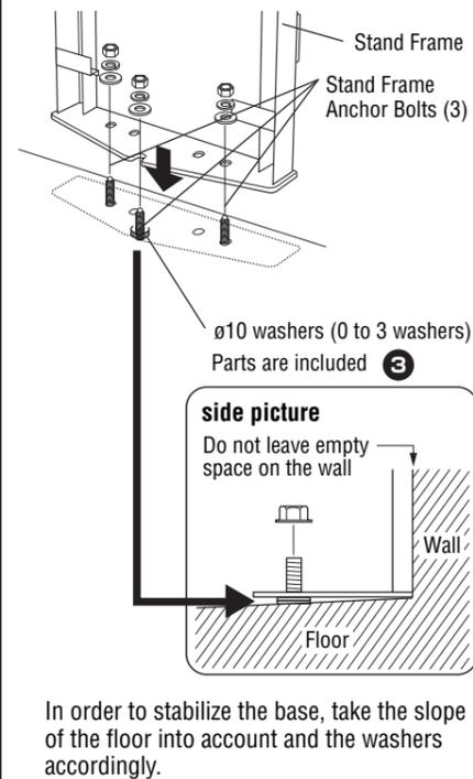
**5-1** Installation in Concrete/ALC walls. Drive in M6 anchors and fix the unit in place.
