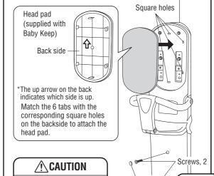
Screw caps, 2 The head pad tabs will (supplied with make a clicking sound Baby Keep) when correctly attached. Note that the tabs may break if forcibly inserted.
