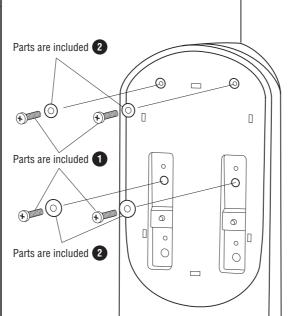
Attach the head pad. (Make sure the correct side is up.)
