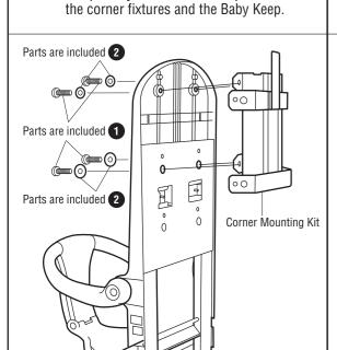
Temporarily place the connected corner fixtures and base in the corner against the wall, and mark the installation points on the wall.
